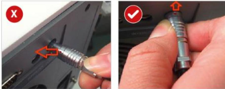
Insert the standard footswitch and interlock connectors with the red dot facing upwards.
