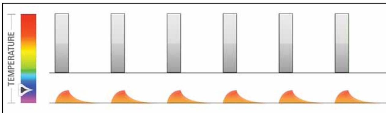
Figure 2. Micropulse technology finely controls the thermal elevation by chopping a conventional mode laser beam into a train of repetitive short pulses, allowing tissue to cool between pulses and reducing thermal buildup.
