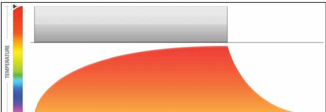
Figure 1. In conventional mode photocoagulation, a rapid rise in the temperature of the target tissue creates blanching and a high thermal spread.
