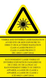
$\begin{array}{ll} \lambda = 810 \text{ nm} & \text{Po} = 3 \text{ W} \\ \lambda = 635 \text{ nm} & \text{Po} = 1 \text{ mW} \end{array}$
